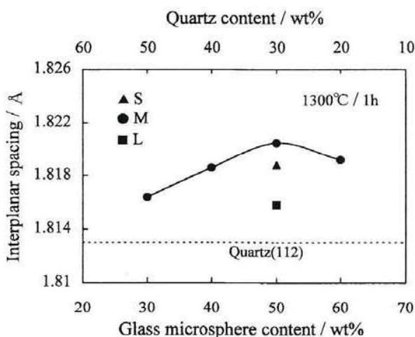
Fig. 7. Interplanar spacing of quartz (112) plane with various compositions and quartz particle size in fired bodies. --- Quartz (112) standard.
