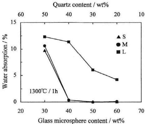
Fig. 6. Change of water absorption in fired bodies.
