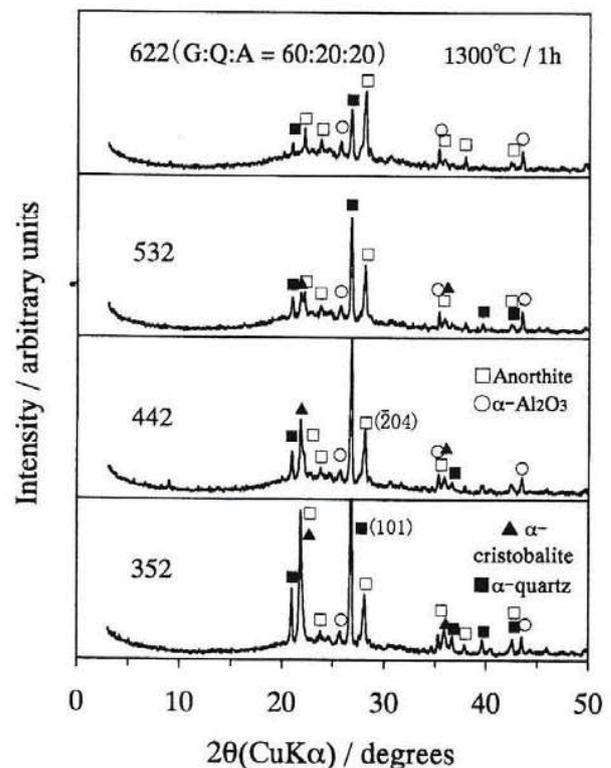
Fig. 3. XRD patterns with various compositions and M quartz particle size in the fired bodies. G, Glass microsphere; Q, Quartz; A, Aluminous cement.
