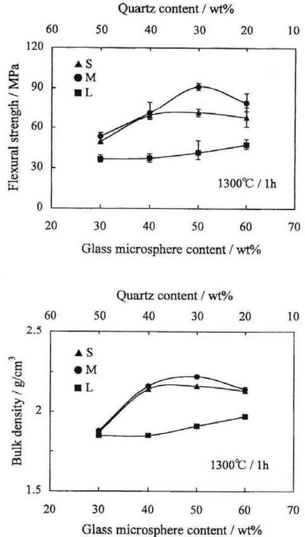
Figs. 4 and 5. Change of flexural strength and bulk density with various compositions and quartz particle size in fired bodies.
