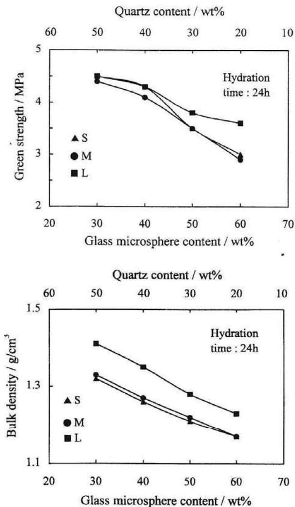
Figs. 1 and 2. Variation of green strength and bulk density as function of composition and quartz particle size in green bodies.
