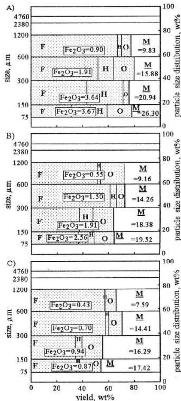
A)5000gauss,B)10000gauss,C)15000gauss, F,H,O: nonmagnetic (F: feldspar, H: hornblende, O: quartz, mica, etc.), M: magnetic, Fig. 6. The yield and Fe<sub>2</sub>O<sub>3</sub> content of separated fractions.
