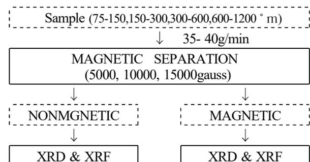
Fig. 2. Process flowchart for magnetic separation
