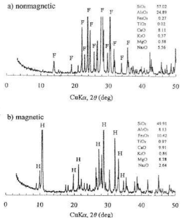
Fig. 4. X-ray analysis of separated products.
